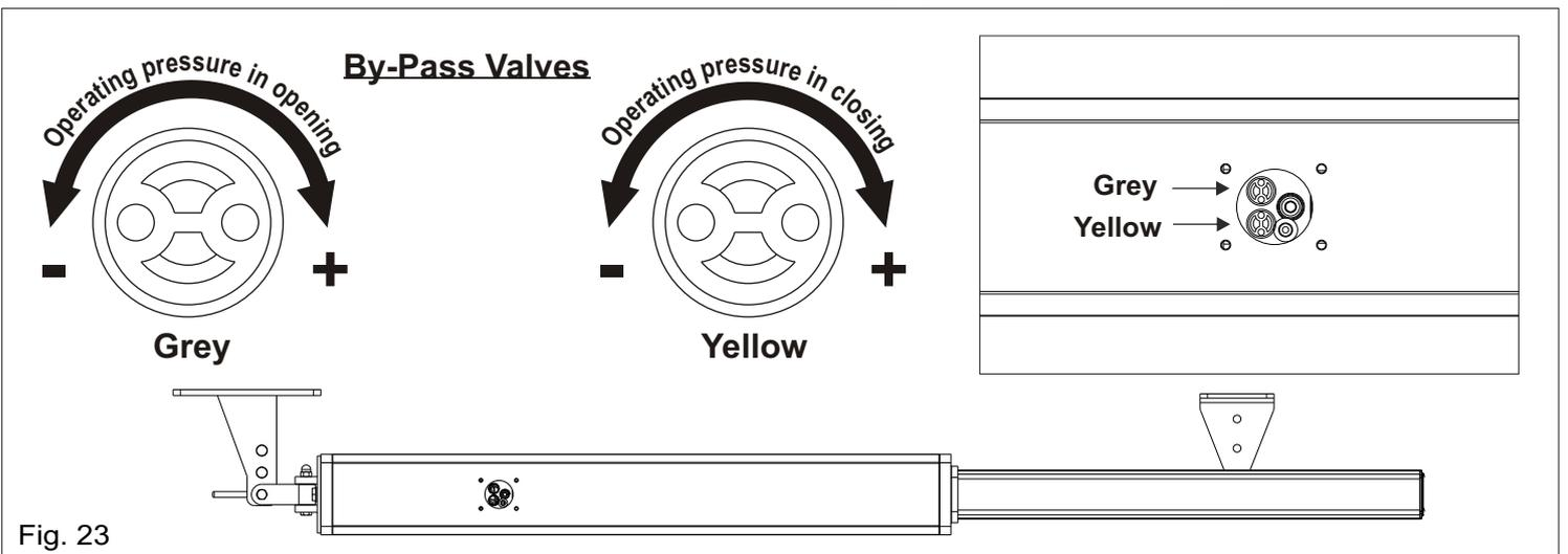
Adjust the opening and closing forces of the gate so that the diagram of the force is respected (present in the regulation EN 12453); Anyway the max. thrust force should never be superior of 15 kgF.
