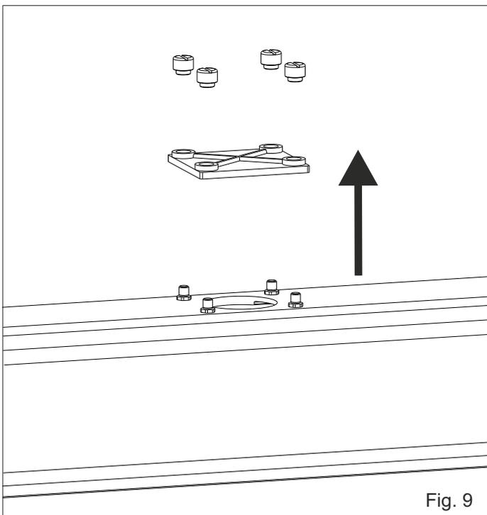
Remove the transporting plate as shown in Fig. 9
